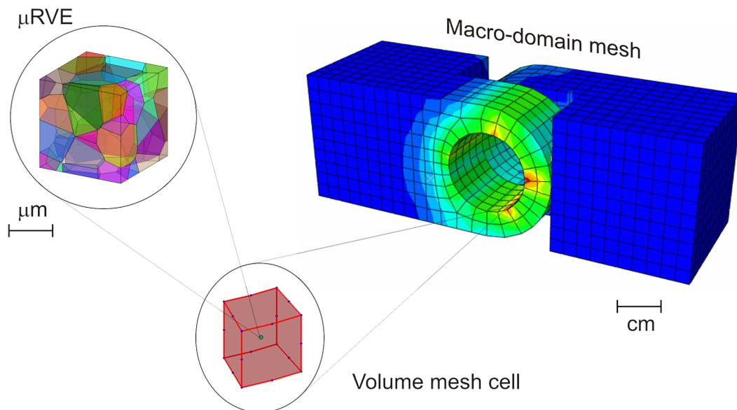
**Fig.1:** A schematic illustration of multiscale modeling of polycrystalline components.
