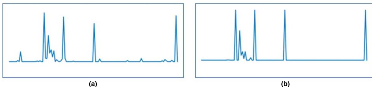
**Figure 5:** Illustration of reconstructed network traffic sample (b) by the proposed DAE network from the original 1D network traffic (a)
